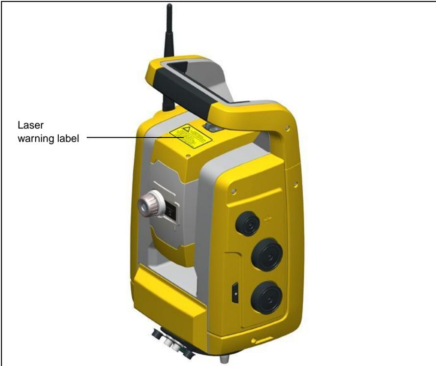
Figure 3.4 Location of laser warning label on a Trimble S3 Total Station
