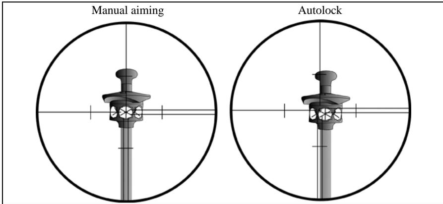
Figure 5.35 Difference between aiming manually and Autolock
