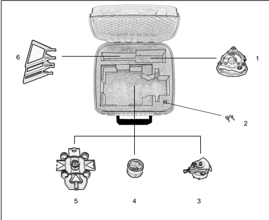
Figure 6.46 Contents of the traverse kit 1 accessory case
