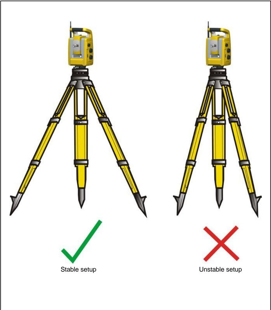
Figure 5.37 Tripod setup
