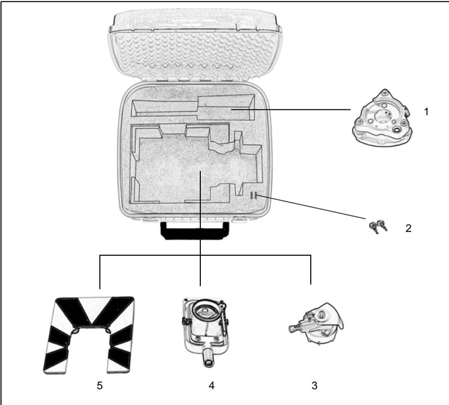
Figure 6.48 Contents of the traverse kit 2 accessory case
