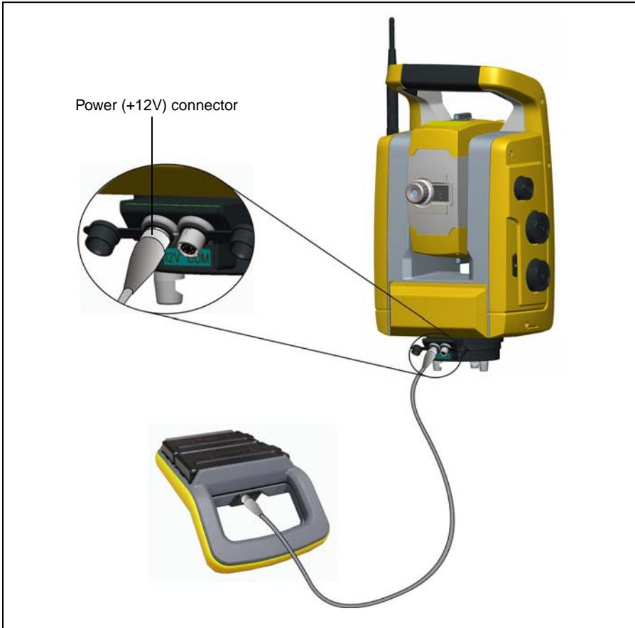
Figure 3.16 Connecting the Multi battery Adapter
