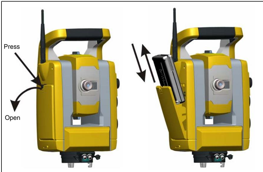
Figure 3.14 Removing and replacing the internal battery
