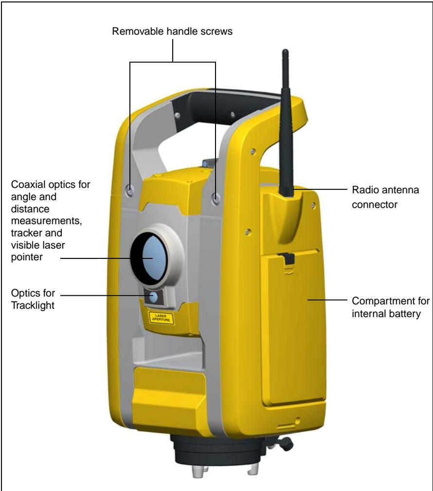
Figure 3.9 Front view of the Trimble S3 Robotic Total Station
