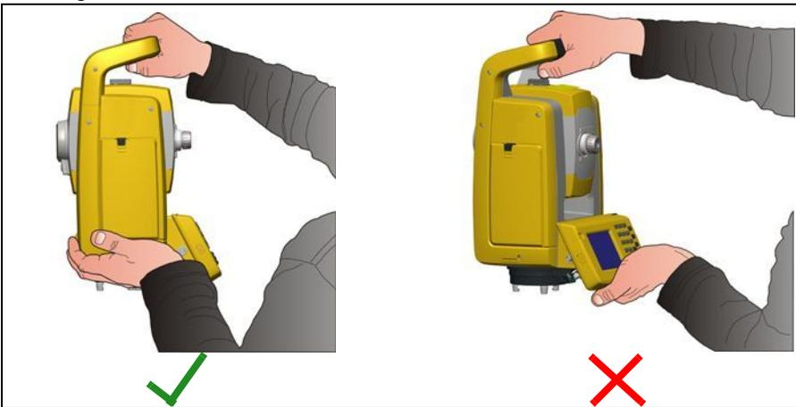
Figure 2.2 Lifting the Trimble S3 Servo/Autolock Total Station.
