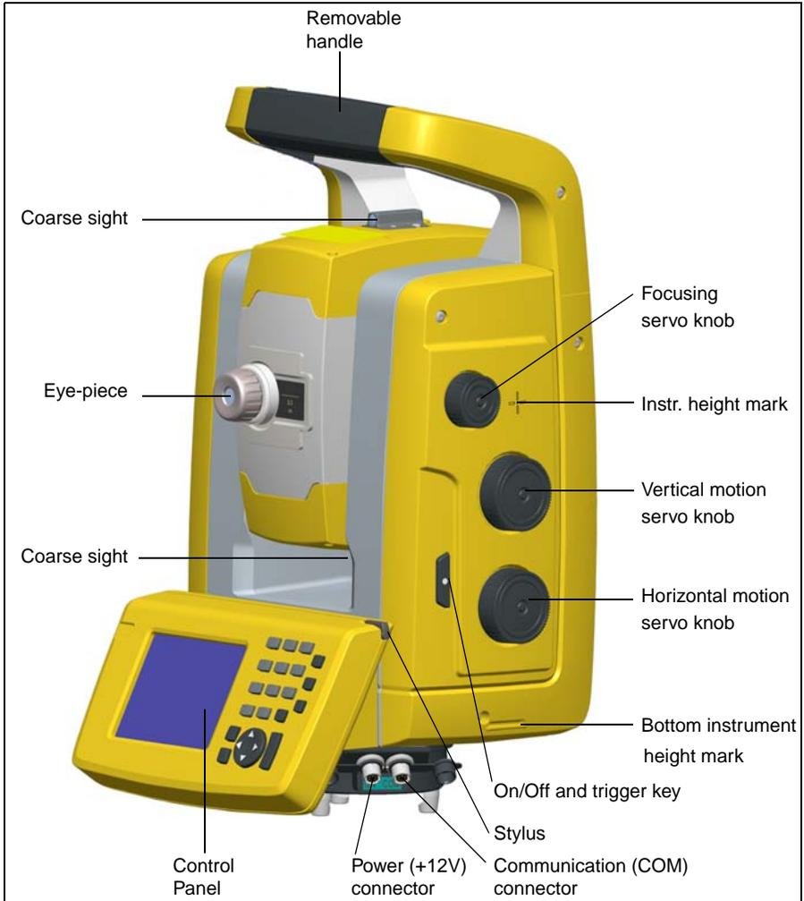
Figure 3.10 Operator's view of the Trimble S3 Servo/Autolock Total Station
