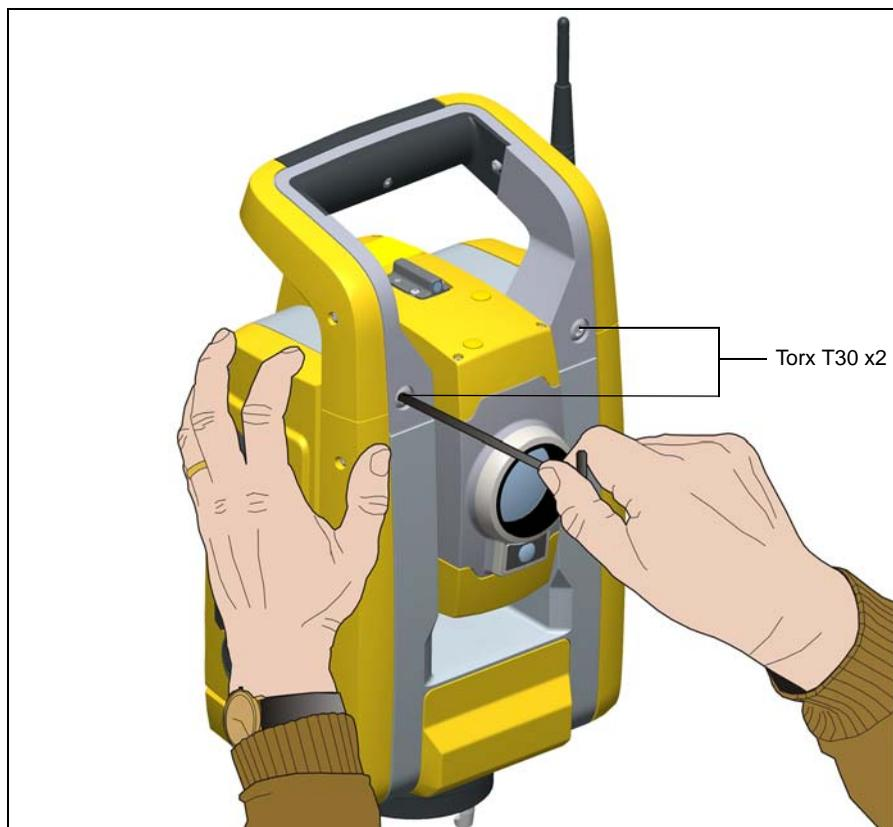
Figure 5.43 Removing the Trimble S3 Total Station handle
